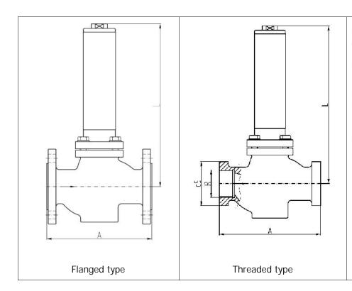
The pressure relief valve S3 model works with direct action principle.
